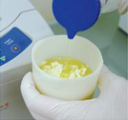
1. Add alginate powder and water into the mixing cup.
