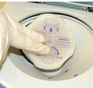
3. Put the mixing cup into the mixing well.
