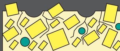
Mechanical stress concentrates on surface voids leading to crack propagation
